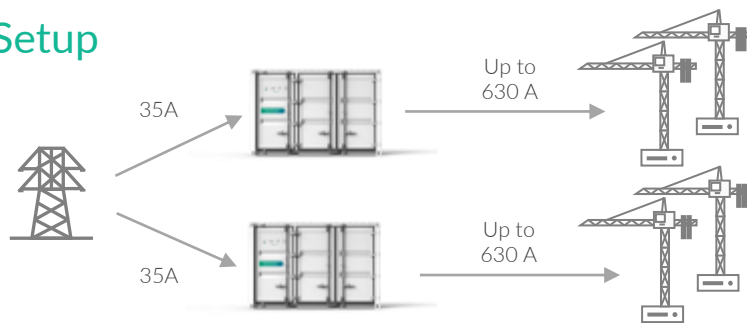
Figure 1. 'Block' diagram of the connection between the utility mains, Enertainers and the loads.
